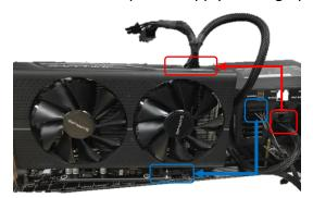
Step 4. The first mining kit (PCIe riser + graphics card + power connections) should be installed on slot PCIE2. That is the x16 slot.
